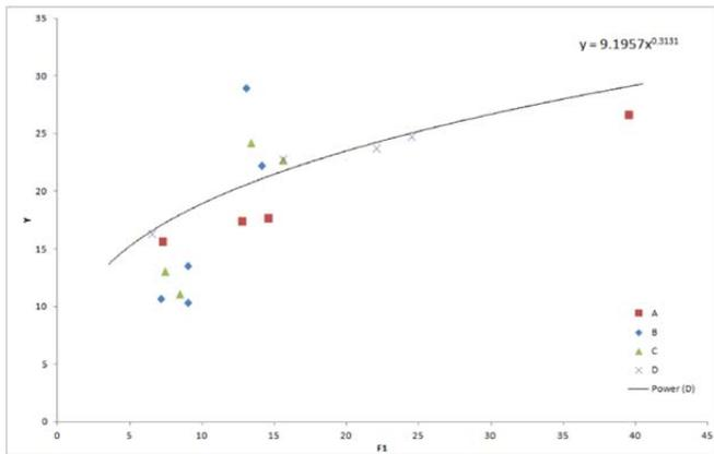
Fig. 9: Sequent depth versus initial Froude number
