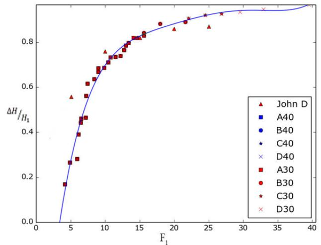
Fig. 7: Relative energy loss versus Initial Froude number
