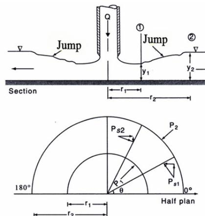
Fig. 1: Definition Sketch for Radial Hydraulic Jump
