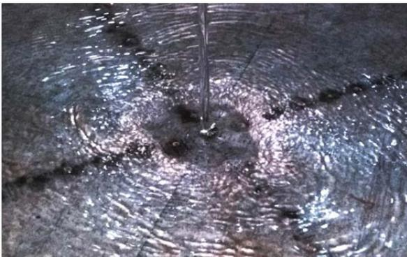
Fig. 5: Symmetrical jump at lower discharge
