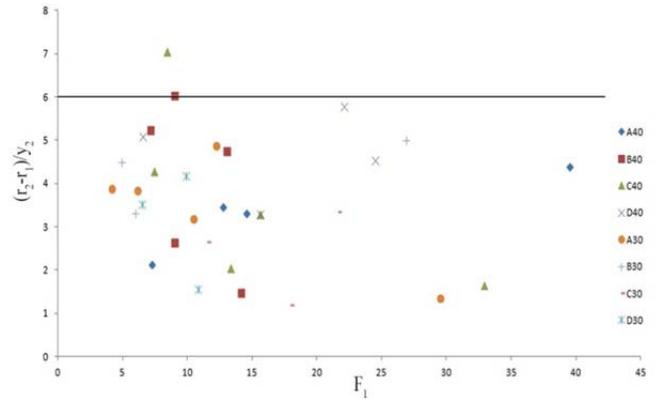
Fig. 10: Jump length ratio versus initial Froude number
